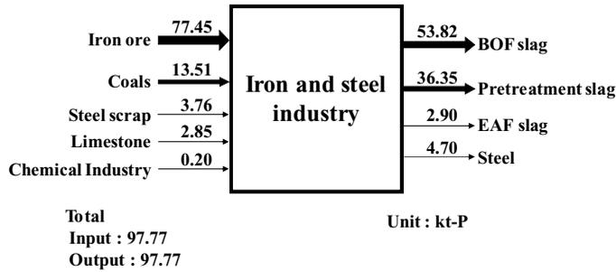
**Figure 9** Phosphorus flows associated with the iron and steel industry, in kilotons of phosphorus (kt-P). BOF = basic oxygen furnace; EAF = electric arc furnace.
