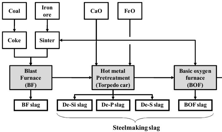
**Figure 16** Schematic process flow diagram of the conventional BF–BOF steelmaking process, where silicon, phosphorus, and sulfur in molten pig iron (hot metal) are removed by the hot-metal pretreatment process before charging to the BOF. BF = blast furnace; BOF = basic oxygen furnace; De-Si = desilicization; De-P = dephosphorization; De-S = desulfurization; CaO = calcium oxide; FeO = iron oxide.
