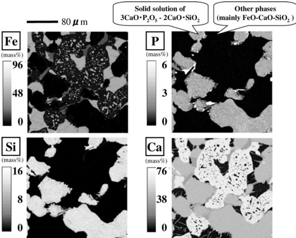
**Figure 17** EPMA (energy-dispersion type electron-probe microanalysis) mapping image of a dephosphorization slag ( $\text{Fe}_t\text{O} = 19\%$ ,  $\text{CaO}/\text{SiO}_2 = 4.4\%$ ,  $\text{P}_2\text{O}_5 = 2.8\%$ ) supplied by a Japanese steelmaking company.
