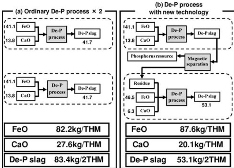
**Figure 18** Recovery of phosphorus by magnetic-separation technology, in kilograms per ton hot metal (kg/THM). CaO = calcium oxide; FeO = iron oxide; De-P = dephosphorization.
